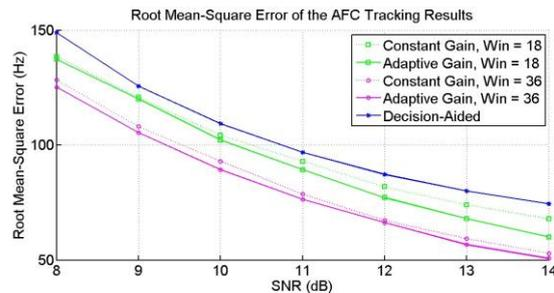
Fig. 6. Comparison of convergence speed with different settings.
