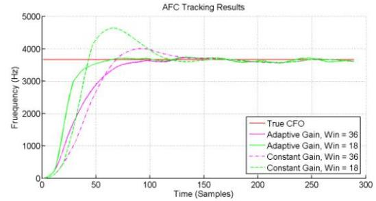
Fig. 4. Tracking logs of the AFC with different settings.
