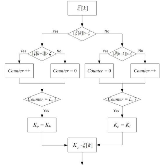
Fig. 3. Flow chart of automatic gain control.
