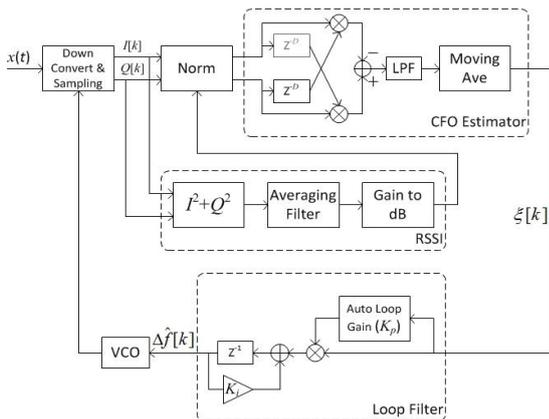
Fig. 1. Block Diagram of the Proposed AFC.
