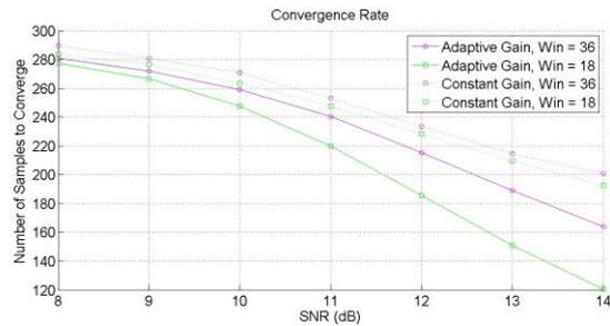
Fig. 5. Comparison of convergence speed with different settings.
