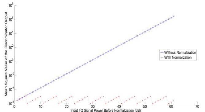
Fig. 2. Discriminator output of the normalized I Q samples.
